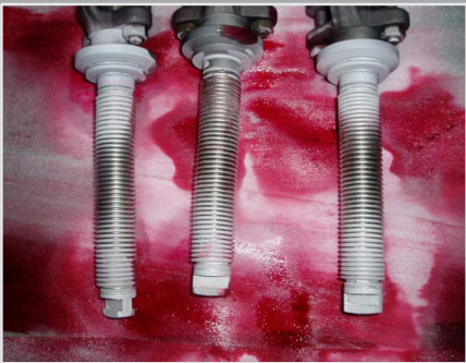
Post cycling penetrant test of bellows
