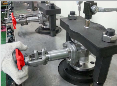
Pressure testing of each valve
