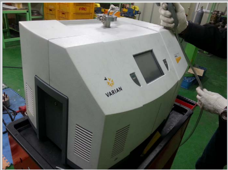
Helium leak testing – instrument sensitivity < 10^{-3} \text{ mm}^3/\text{s}
